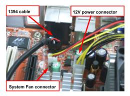
4. Disconnect the P1 power cable and ODD data cable from the main board.
